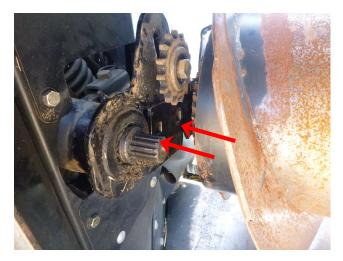
6. Remove the 2 mount bolts on the RH side.
