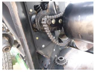
(Endless chains will need to be fitted to the Drum Sprocket and Drive Shaft Sprocket on Drive Shaft before fitting bolts to Mount Arm on LHS)
