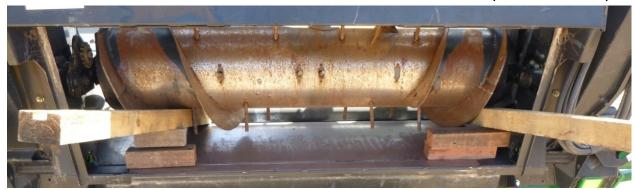
5. Remove the 2 mount bolts on the LH side.
