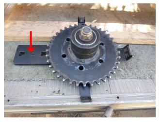
2. Fit Mount Arm Assembly to Turbodrum with 6 Bolts from supplied sprocket.
