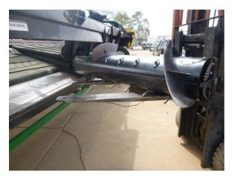
5. Slide the TurboDrum off the forks into the front with the RHS going in first.
