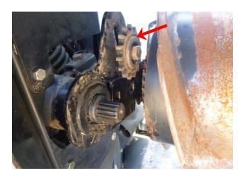
3. If you have an endless chain you will need to slide the drive sprocket off the drive shaft
