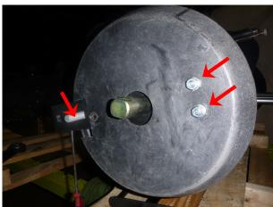
9. Fit Finger Timing Plate to RH end with round boss through Plastic Cover.
