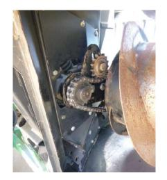
2. Remove the Idler Sprocket and Drive Chain.
