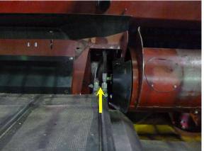
7. Mark position of top stoppers and remove from RH & LH side of drum.
