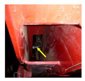
11. Remove RH main pivot bolt on arm.
