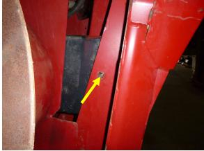
9. Fit LH and RH top stopper bolts to old marks and tighten.
