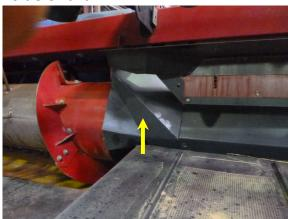
6. Remove hydraulic hoses from LH & RH belt hydramotors.
