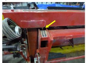
3. Remove drive shaft from LH side of drum
