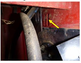
10. Tighten the 4 LH mount arm bearing flange bolts and ensure bearing is locked to shaft.
