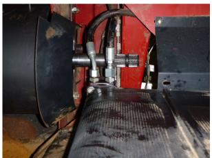
5. Fit PTO drive shaft to LH side.
